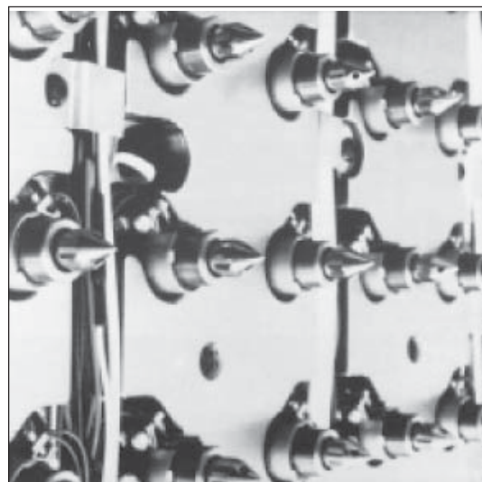
PROTHERM is especially recommended for nozzle tips, edge gates and manifold in hot runner systems.
